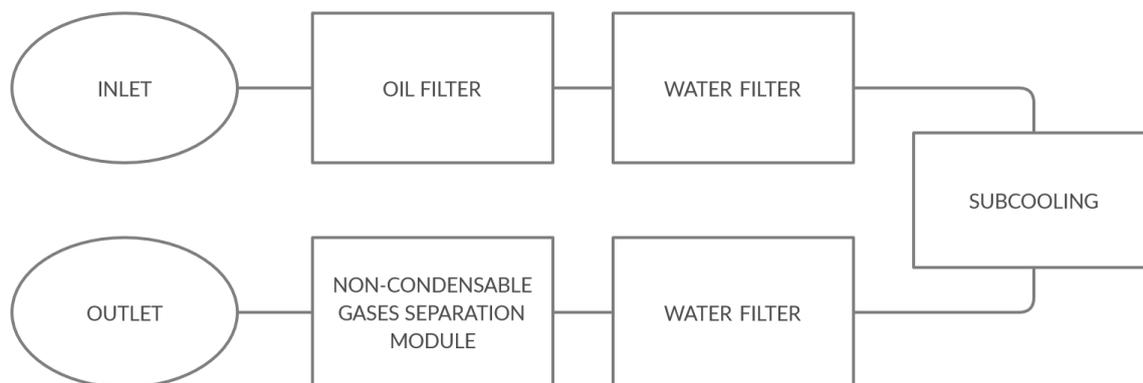
Figure 1. Block diagram of refrigeration reclamation machine.
